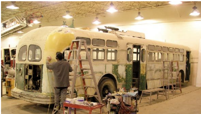
Left: 9631 being sanded on 9 February in preparation for painting.
